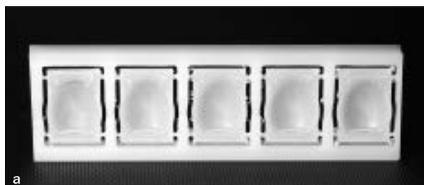
Fig 1 Test implant made of medical UHMW-PE. (a) Series of prefabricated implants. (b) Final test implant.
