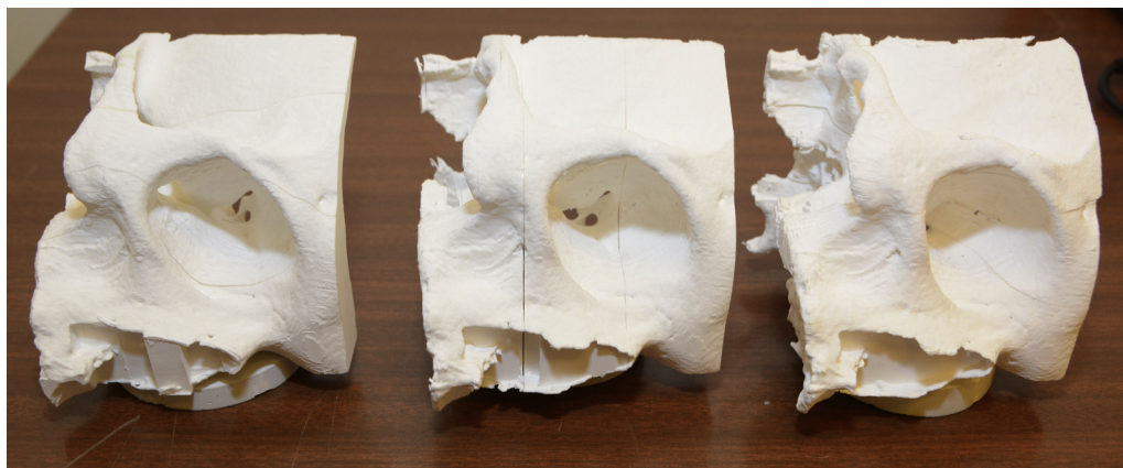
Fig. 2. Paper-based models printed on a Matrix 300 3D printer. Each model consists of three smaller parts, which were printed separately and later stuck together with glue. From the left, the models are cut in the coronal, axial, and sagittal planes.
