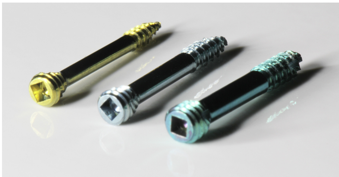
Fig. 1. The proposed set of small-diameter compression screws (all 14 mm long) that can be completely embedded in bone for rigid internal fixation of the condylar head of the mandible. Left: outer diameter of leading thread = 1.5 mm, shaft = 1.1 mm in diameter; middle: outer diameter of leading thread = 1.8 mm, shaft = 1.4 mm in diameter; right: outer diameter of leading thread = 2.0 mm, shaft = 1.6 mm in diameter.
