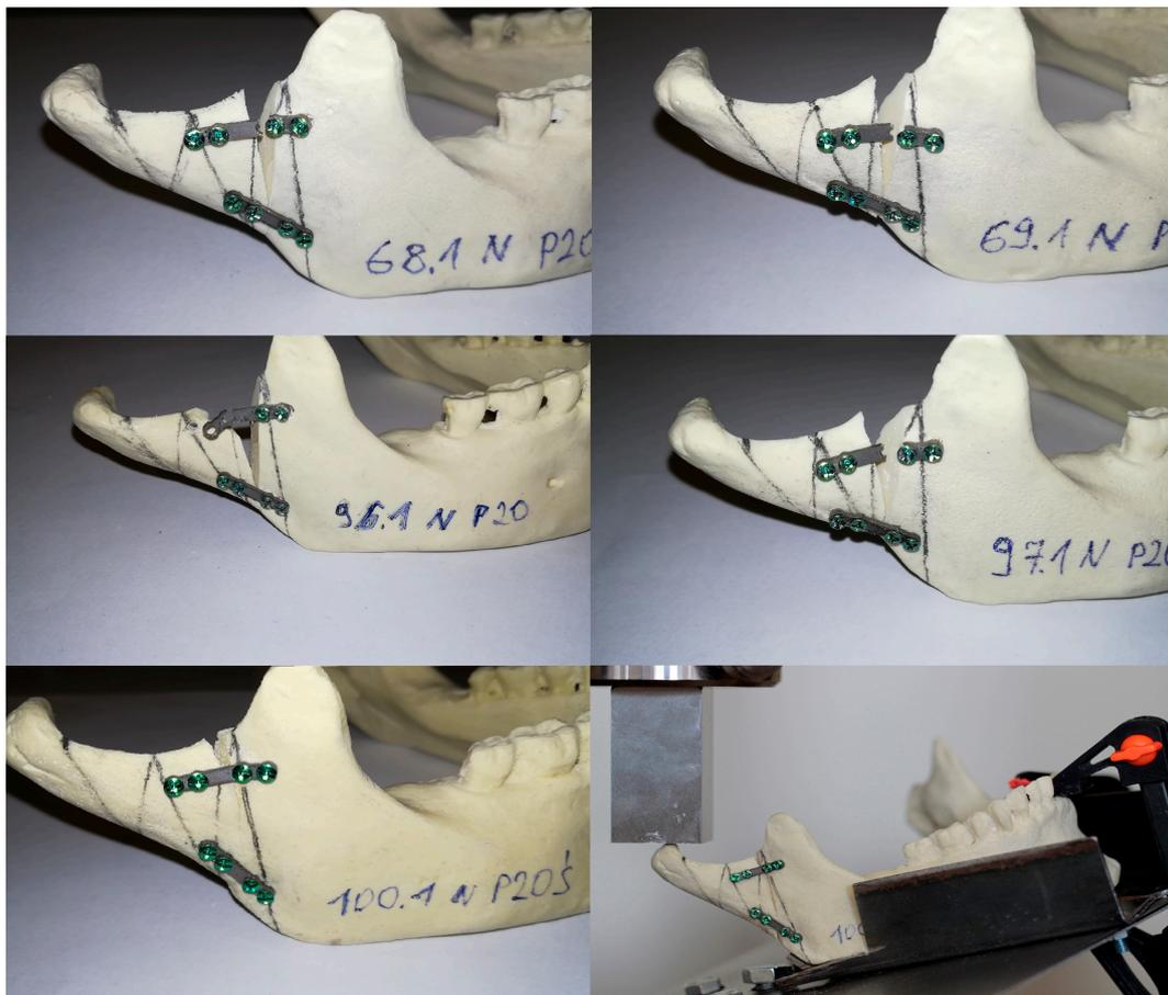
**Figure 1.** 5 samples of polyurethane mandibles with broken plates number 20 and 1 sample of mandible on testing plate in the testing machine.
